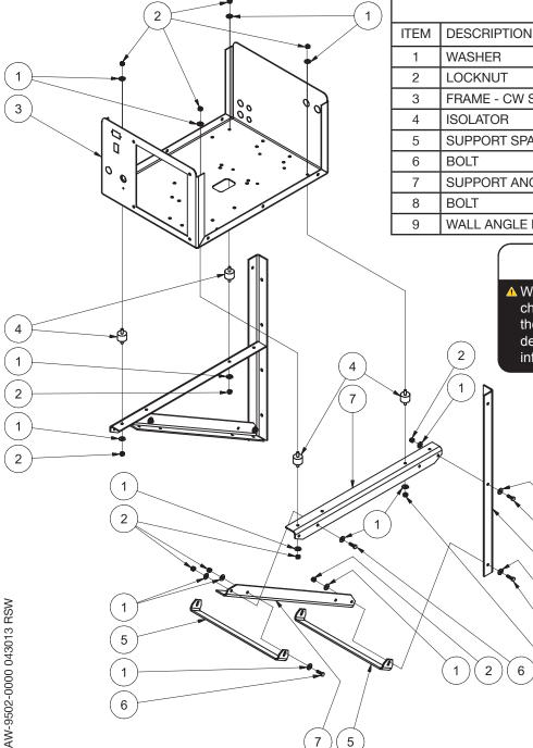
PART # QTY 28-0022 24 30-0157 16 FRAME - CW STATIONARY - SS 1 21-0193 33-0028 4 SUPPORT SPACER BRACKET 20-0777 2 27-0067 6 SUPPORT ANGLE 4 20-0776 27-0068 2 WALL ANGLE BRACKET 20-0775 2
